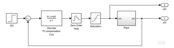
Emulate (discretize) the PI compensator from part 3 using the backward differencing method.
