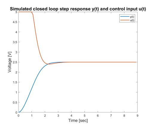
8. Program the observer-based state feedback control for the LMC6484 op amp circuit Insert a fully labeled experimental closed loop step response plot for a 2.5V step reference input, with an overlay of the simulated step response from part 7 Plot both the response y[n] and the control input u[n] on the same figure.
