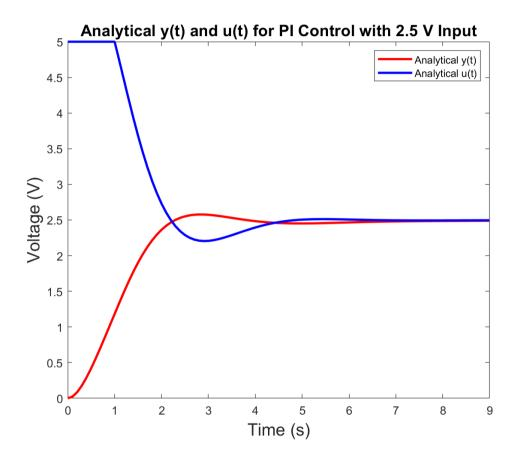
5. Program the discrete PI closed loop control for the LMC6484 op amp circuit Insert a fully labeled experimental closed loop step response plot for a 2.5V step reference input, with an overlay of the simulated step response from part 4. Plot both the response y[n] and the control input u[n] on the same figure.
