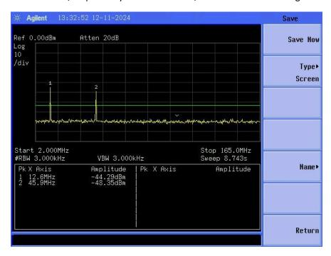
**Spectrum after the second amplifier:** The 0 bit and 1 bit signals still remain at 12.6 MHz and 45.9 MHz, respectively, as shown by peaks 1 and 2. The remaining peaks correspond to distortion products. A second order harmonic around 2\*f1 is found at 24 MHz, and another second order harmonic around 2\*f2 is found at 91.7 MHz.
