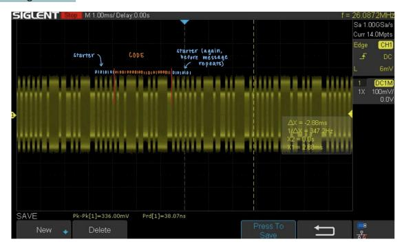
After getting the oscilloscope trace, we first identified which height corresponded to which bit. As given, the frequency for the 0 bit was 2.256 GHz, and that for the 1 bit was 2.296 GHz. The 1 bit corresponds to a higher frequency, but seeing as we were using a low pass filter in our receiver, and these filters attenuate higher frequencies more than lower ones, it was decided that the more attenuated signal (or height) corresponded to the 1 bit.
