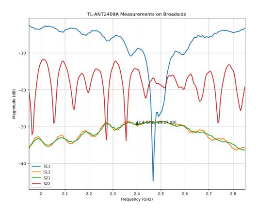
S11 of antenna, extracted from lab 5, because we used the same antenna
