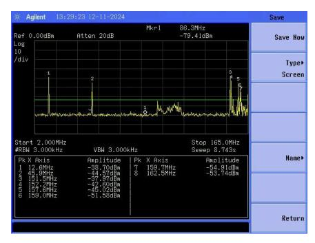
**Spectrum after the low pass filter:** The low pass filter had a cutoff at 40 MHz, so the 0 and 1 bit signals weren't affected. Peaks 1 and 2, which correspond to the 0 and 1 bit signals, are still found at 12.6 MHz and 45.9 MHz, respectively. Due to the filter, the blocker and WiFi signals are fully attenuated.
