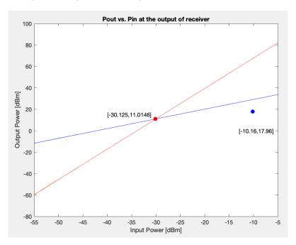
Plot of Pout vs. Pin showing the fundamental power (blue line), the IM3 power (red line), measured IP3 point (in red), and theoretical IP3 point (in blue)
